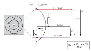
All voltages measured to ground External load resistance Ra from U<sub>A</sub> to U<sub>BA</sub> required.
