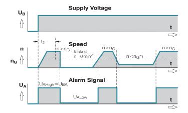
$t_2 = \hbox{Alarm signal suppression during start-up}$
