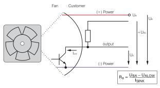
All voltages measured to ground. External load resistance  $R_a$  from  $U_A$  to  $U_{BA}$  required. With VARIOFANs with external temperature sensor for controlling the motor speed, the NTC sensor is not included in the scope of delivery. Temperature sensor LZ 370, see Accessories.
