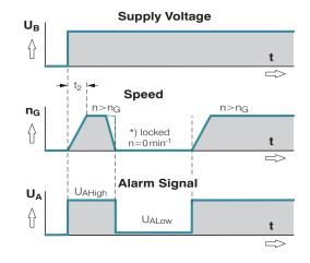
$t_2 = Alarm \ signal \ suppression \ during \ start-up.$
