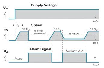
$t_2 = Alarm \ signal \ suppression \ during \ start-up.$
