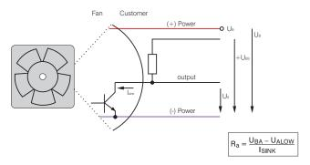
All voltages measured to ground. External load resistance  $R_{\text{B}}$  from  $U_{\text{A}}$  to  $U_{\text{BA}}$  required.
