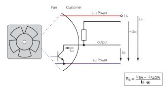
All voltages measured to ground. External load resistance  $R_{\text{A}}$  from  $U_{\text{A}}$  to  $\;U_{\text{BA}}$  required.
