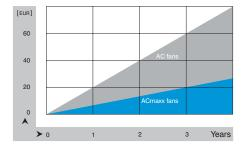
Energy cost comparison: Standard AC fan versus ACmaxx, at the same air performance.
